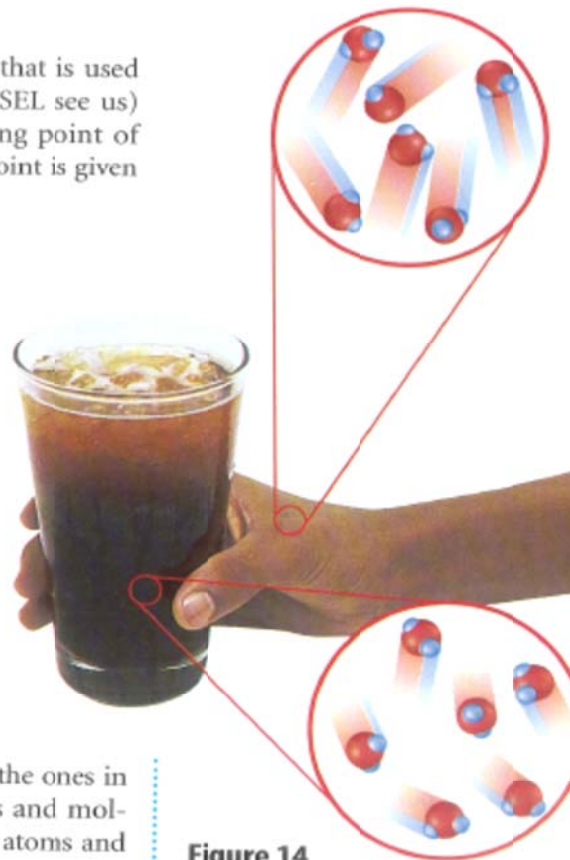
Figure 14 Heat flows from your hand to the glass of iced tea, making your hand feel cold. Why do people wear gloves in cold weather?
